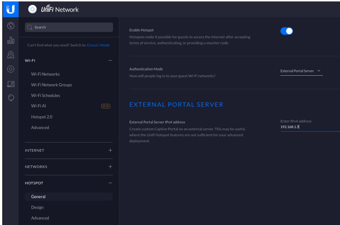
Next, you must allow the device to reach the portal. Go in *Settings* → *hotspot* → *advanced* and configure it as shown below:
